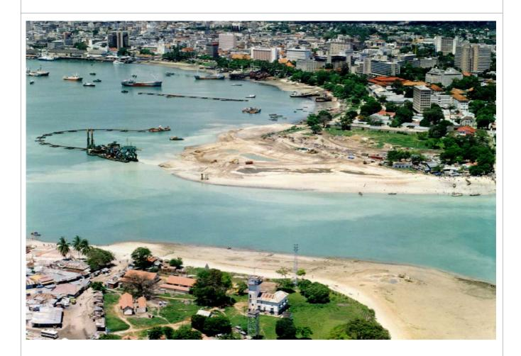
The dredging works to be executed comprised the straightening, widening and deepening of the entrance channel to the Port of Dar es Salaam, including the reshaping of West Ferry Point and dredging of the Inner Harbour.
